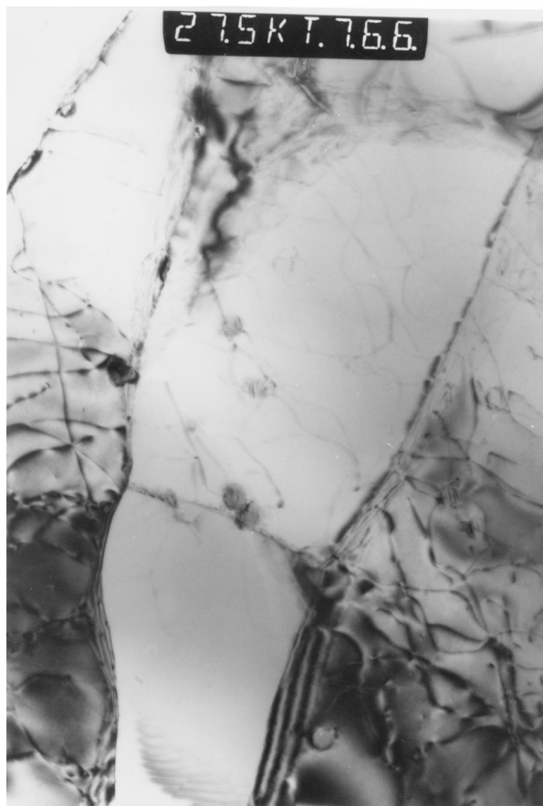
Figure 10 TEM micrograph of Al 6013/SiC interface showing dislocation generations.
